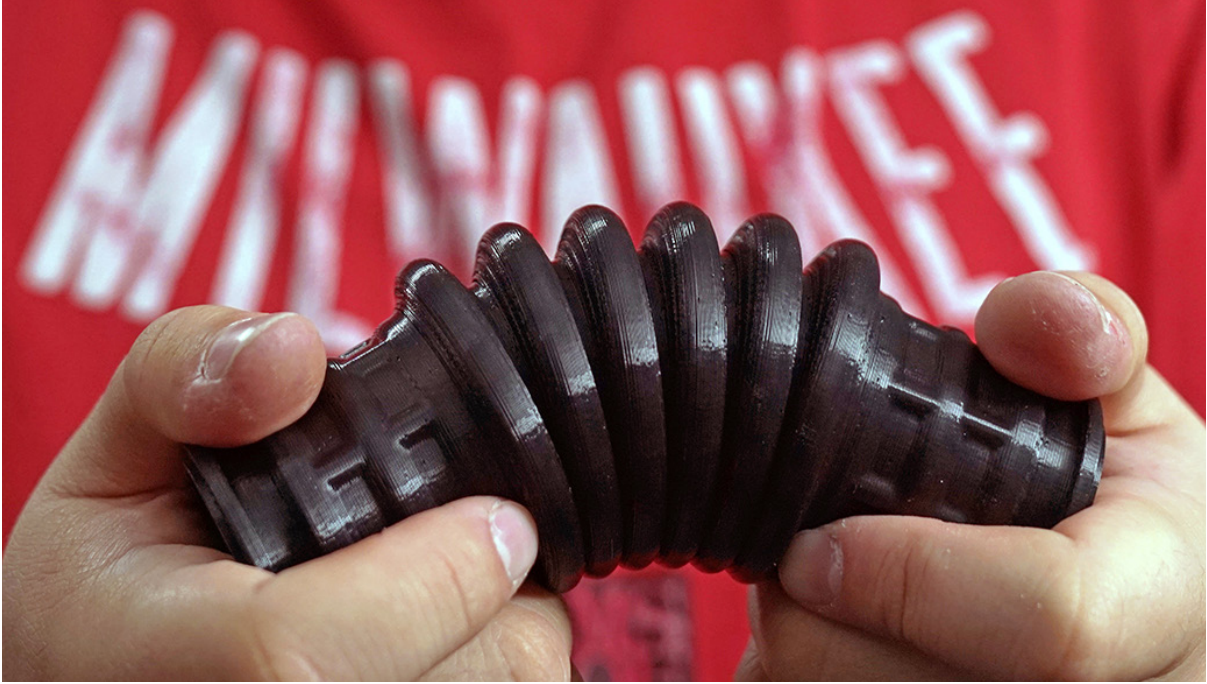
An air intake hose printed in flexible FDM TPU 92A elastomer material.
