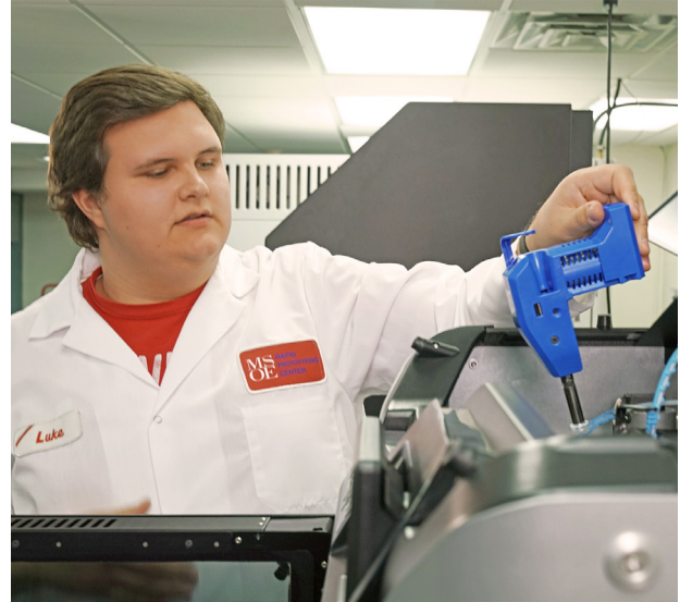
The interchangeable print head enabling easy and fast change-over to elastomer printing.
