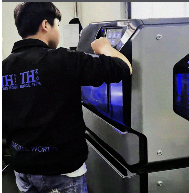
TH Zipper uses the Stratasys J55 to make pullers and buttons prototypes
